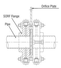
Orifice Assembly with SORF Flange & Flange Taps
